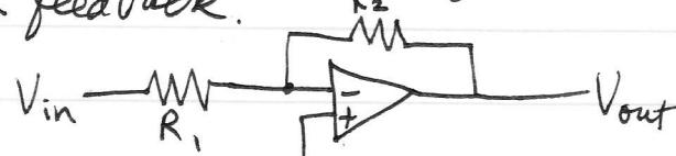
$$\frac{V_{in}}{R_1} = -\frac{V_{out}}{R_2}$$
