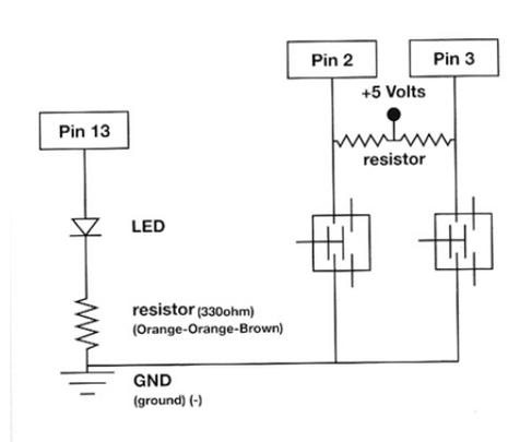
Connect the push buttons, the LED, and the resistors as shown above. Connect a resistor around 330Ω to the LED. Use about 10kΩ for the “pull-up” resistors that connect the switches to +5V. When the button is pushed, the voltage to the Arduino goes LOW it is connected to the other end of the 10kΩ resistor, which is connected to ground when the button is pushed.
