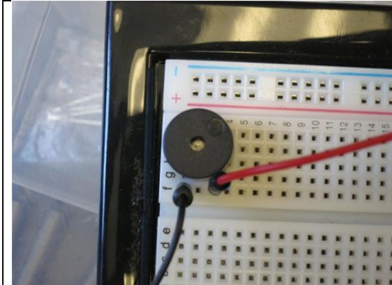
Get a piezobuzzer. Notice that one pin is marked positive. Put it into your breadboard, and connect the positive pin to pin 9 of your Arduino. Connect the other pin to Ground.
